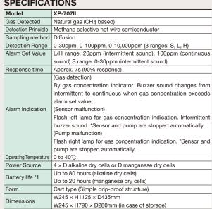
Weight Approx. 4.9 kgs. (including batteries) \*1 Battery life may vary with ambient conditions, conditions of use, storage period, battery manufactures, etc.
