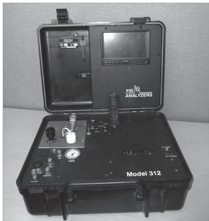
Figure 4.11 – Model 312 person-portable GC, equipped with PID.
