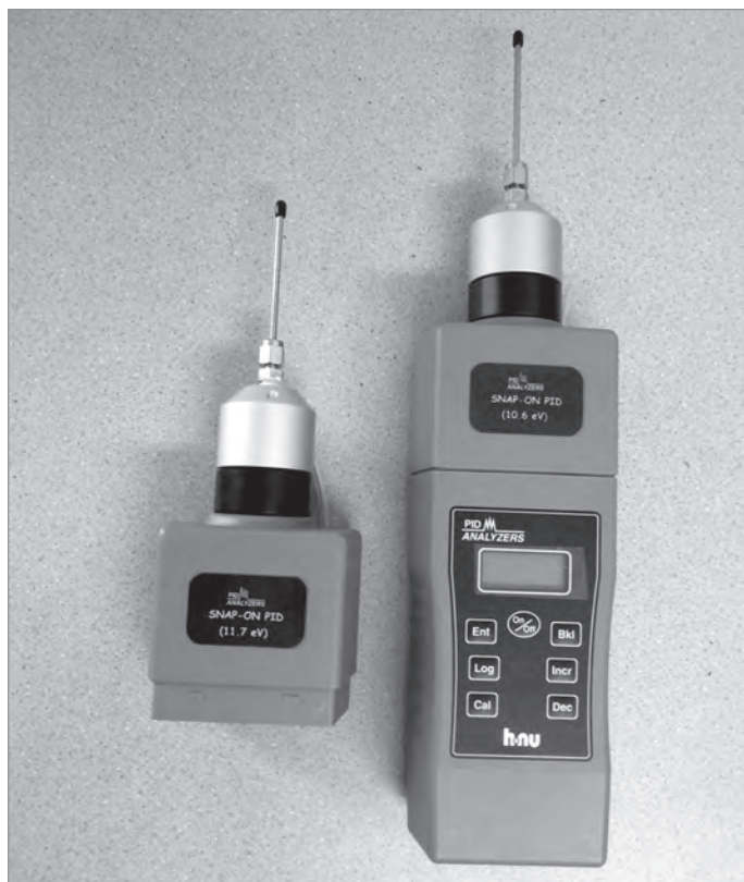
Figure 4.6 – Model 102+ handheld PID (right), with an interchangeable head (left) that may be used to quickly switch between UV lamps of different energy levels. Provided courtesy of PID Analyzers, used with permission.
