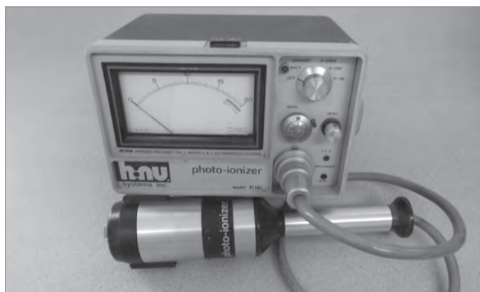
Figure 4.2 – HNU PI101 handheld PID instrument.
